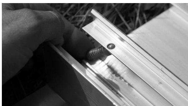
Push the pin in the lower area out of the base by hand (use a screwdriver to help if necessary)
