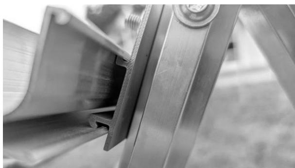
Hook the cable duct into the upper part of the adapter and click it into place by pressing down.
