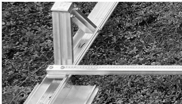
Place the mounting template in the parallel basic sets in the same spot.
