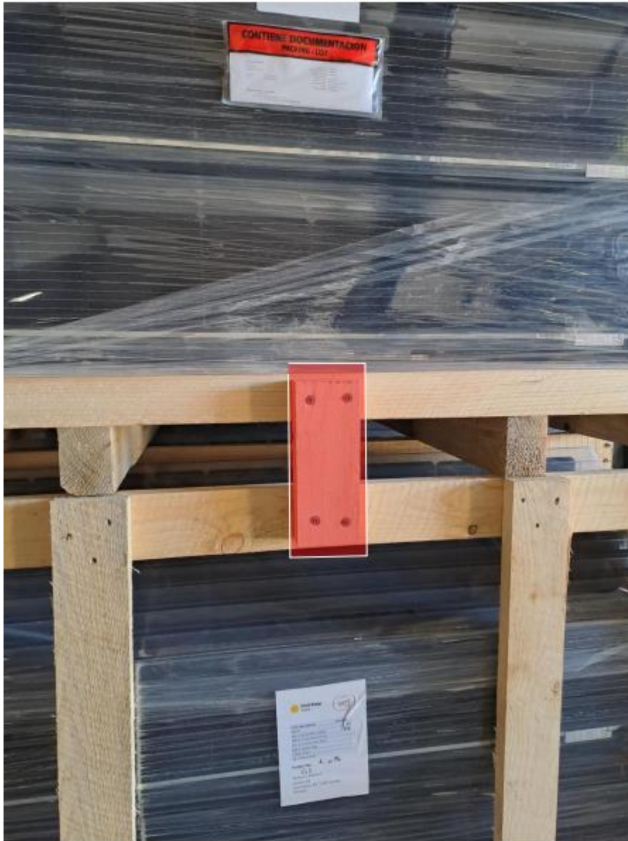
Figure 4: Screws connecting the upper and lower pallets
