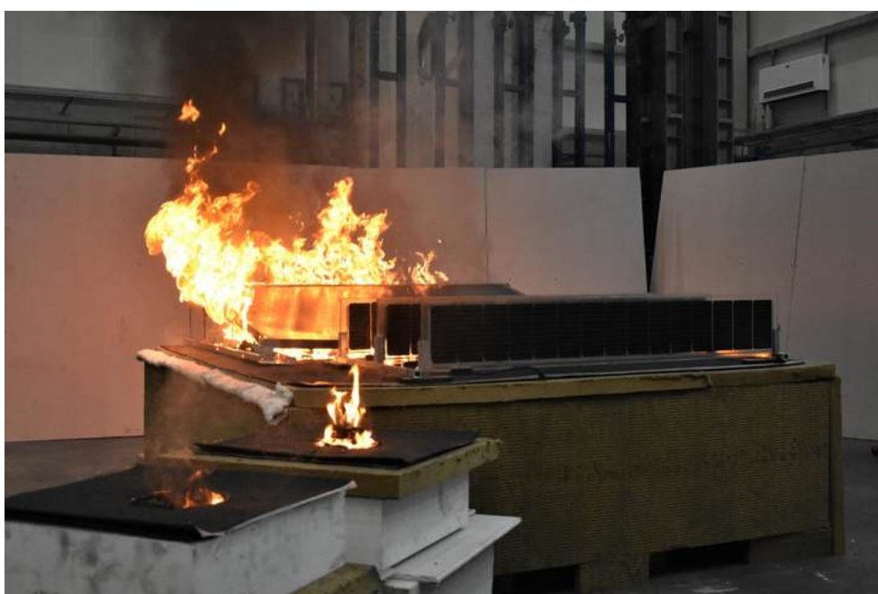
Fire test: Fire spread beneath low-angle panels but was contained with vertical ones.
