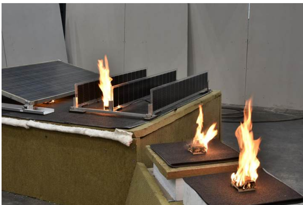
Fire test: Fire spread beneath low-angle panels but was contained with vertical ones.
